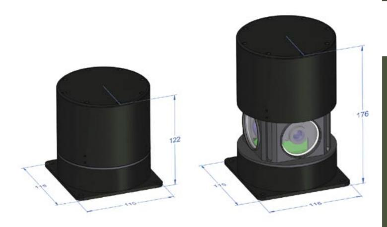
The panoramic camera head is manufactured of aluminum alloy and weights 1680g only. The head is attached to the display unit using single robust Amphenol connector. Ethernet network adapter can be optionally connected to the head instead of the display unit.
